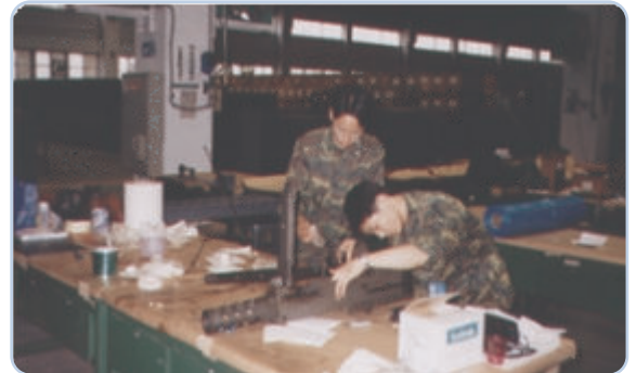
Cleaning and preparation of 0.5 caliber Brownings with Vapro VBCI-818 CLP before preservation.
